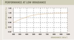
The typical relative change in module efficiency (at nominal power) at an irradiance of 200 W/m² in relation to 1000 W/m² (both at 25  $^{\circ}\text{C}$  and AM 1.5 G spectrum) is -4.0 % rel.
