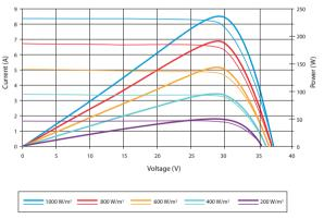
Excellent performance under weak light conditions: at an irradiation intensity of 200 W/m² (AM 1.5, 25 °C), 96% or higher of the STC efficiency (1000 W/m²) is achieved
